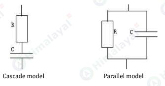
Theoretical cascade model  $tg\delta=2\pi fRC$ , parallel model  $tg\delta=1/(2\pi fRC)$ , R and C basically stay the same, f is a variate. Substitute 45Hz, 50Hz, 55Hz respectively into the formula, draws the conclusion that  $tg\delta$  turns proportional and inverse over frequency f. As shown on the diagram below, f has greater impact on fully proportional and fully inverse model.
