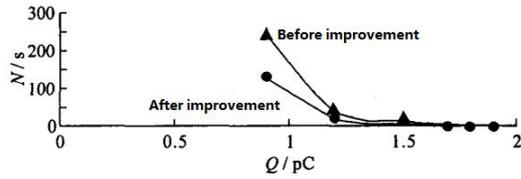
Fig.4 Comparison curve of  $Q_n$  before and after-improvement
