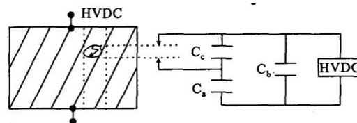
Fig.1. Model of air gap discharge in the medium
