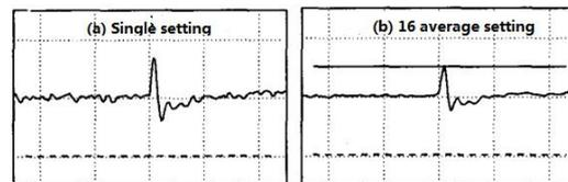
Fig.3 Output waveform at different sampling setting
