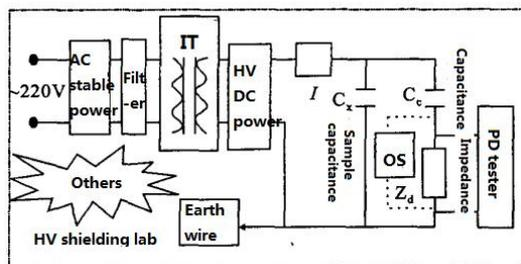
Fig.2 PD discharge circuit
