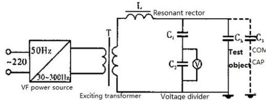
Fig.1 Wiring of series variable frequency resonant test
