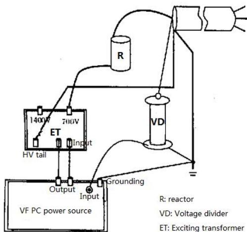
Fig.3 Wiring of single reactor, low voltage and medium/short cable test
