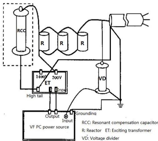
Fig.2. Wiring of three parallel reactors, low voltage and long cable test
