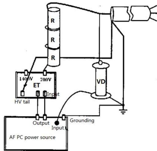
Fig.4 Wiring of three series reactors and short cable or HV cable test
