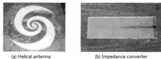
Fig.4 Ultra-high frequency sensor
