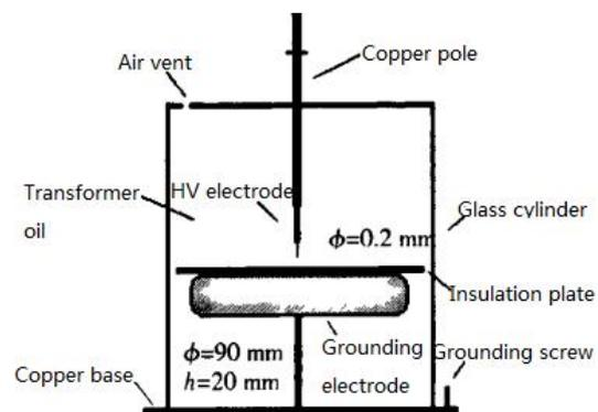
Fig.7 Oil-paper needle-plate discharge
