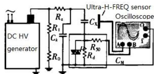
Fig.1 PD test and measuring circuit at DC
