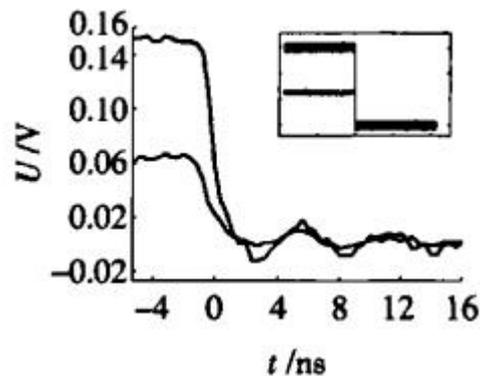
Fig.3 Calibrated impulse and impulse which is transmitted through the measuring system
