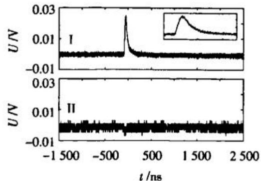
Fig.6 Corona discharge waveform and ultra-high frequency signal
