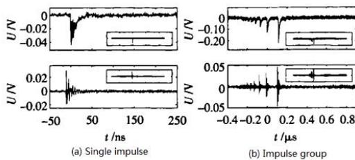
Fig.8 Oil-paper needle-plate discharge impulse waveform and ultra-high frequency signal
