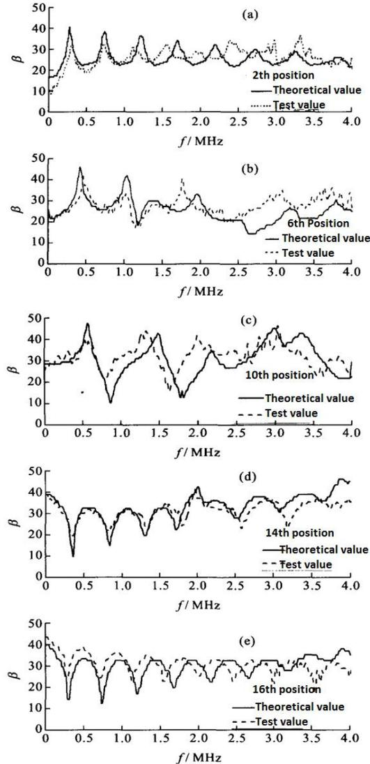
Fig.4 Comparison of theoretical and test values of current transmission function in different positions
