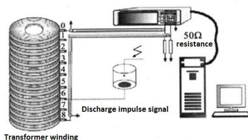
Fig.3 Measurement system for transformer winding current transmission function
