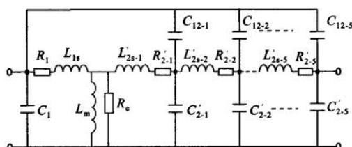
Fig.5 Equivalent circuit of transformer
