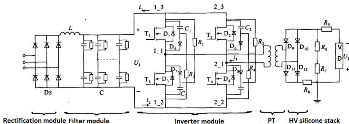
Fig.2 Main circuit diagram
